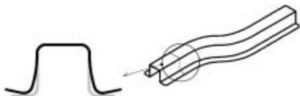
Fig.1 Side-wall Warp of Stamping Parts (1)
